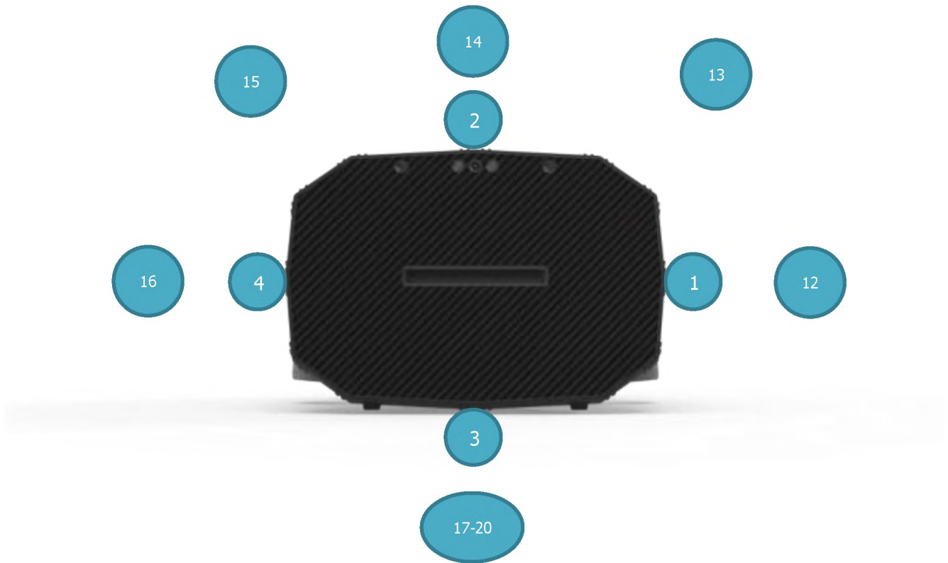
Figure 5: Measurement Locations – Front Detector Vertical Plane
