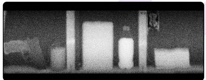
WALL - LEFT TO RIGHT: GUN, EXPLOSIVES, DRUGS, LIQUID, LISTENING DEVICE AND CASH DETECTED
