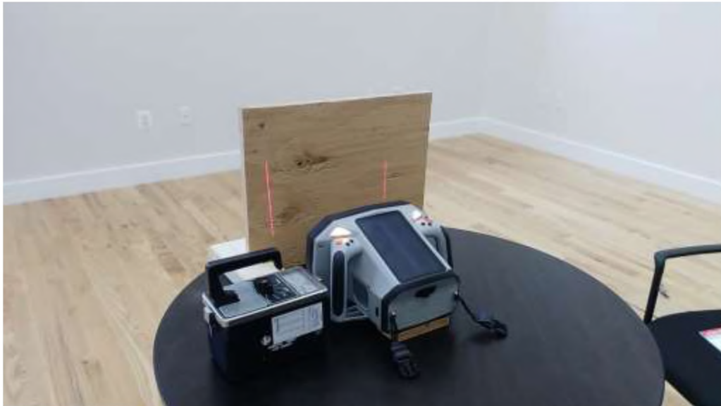
Figure 8: Scatter/Leakage Measurements with 3/4" Plywood at 10 cm
