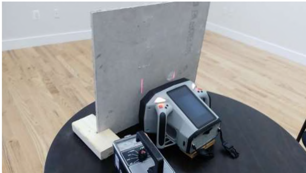
Figure 9: Scatter/Leakage Measurements with 3/8" Concrete Backerboard at 5 cm
